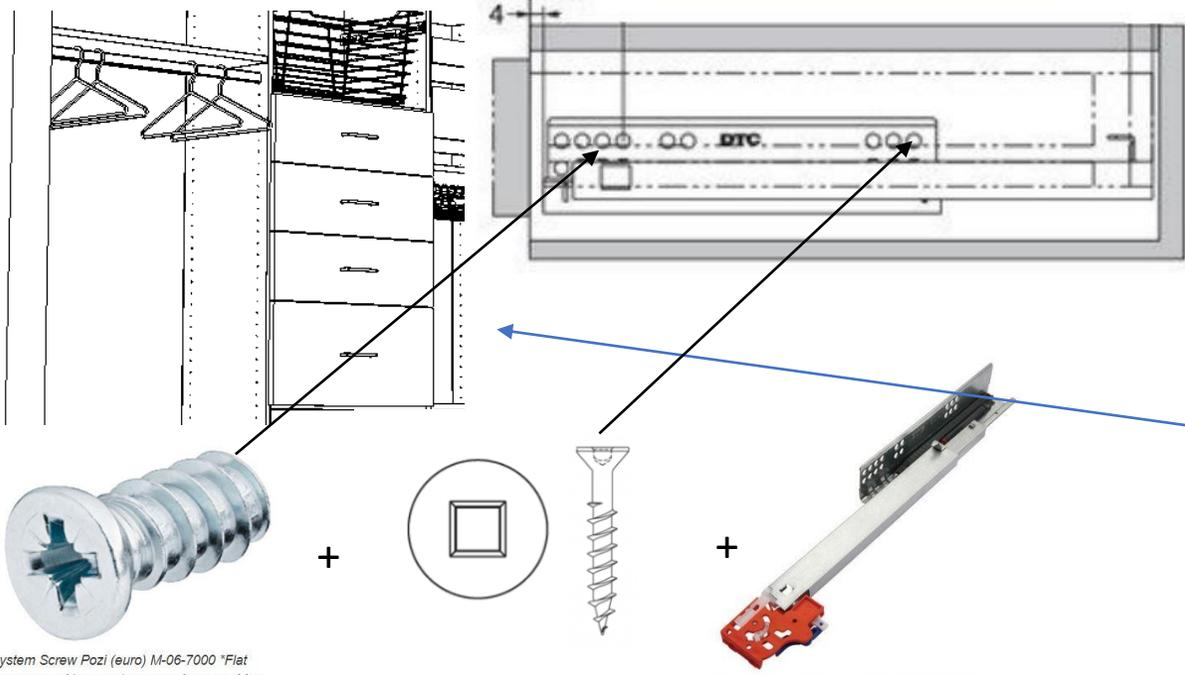
System Screw Pozzi (euro) M-06-7000 \*Flat Screws used to mount accessories on gables
